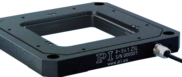
P-541 series nanopositioning Z-stages and Z-tip/tilt stages offer travel ranges of 100 \mu\text{m} with sub-nanometer resolution. They feature a very low profile of 16.5 mm and a large 80 x 80 mm aperture. Versions with strain gauge and capacitive position feedback sensors are available
